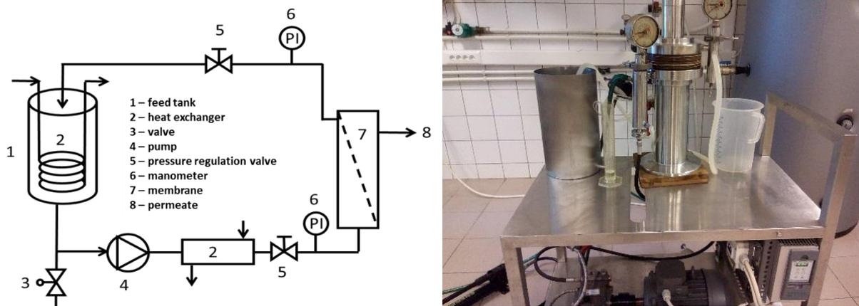
**Figure 2.** Flow sheet and picture of reverse osmosis equipment
