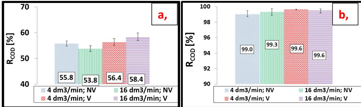
**Figure 3.:** Chemical oxygen demands rejections of (a,) 10 kDa UF membrane (b,) 240 Da NF membrane
