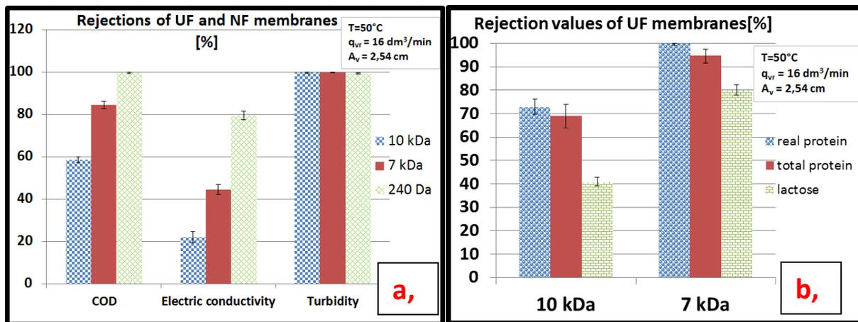
**Figure 3.:** Rejection values measured calculated for different UF and NF membranes
