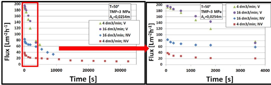
Figure 1.: The impact of vibration and recirculation flow rate on nanofiltration fluxes
