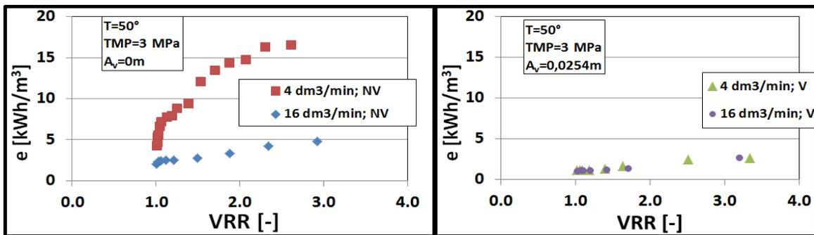
Figure 2.: Specific energy demands in low and high recirculation flow rate experiments, (a) *NV* mode (b), *V* mode.
