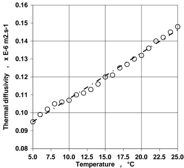
**Figure 5 Relation of perga thermal diffusivity to temperature during the temperature stabilisation in temperature range (5 – 25) °C**
