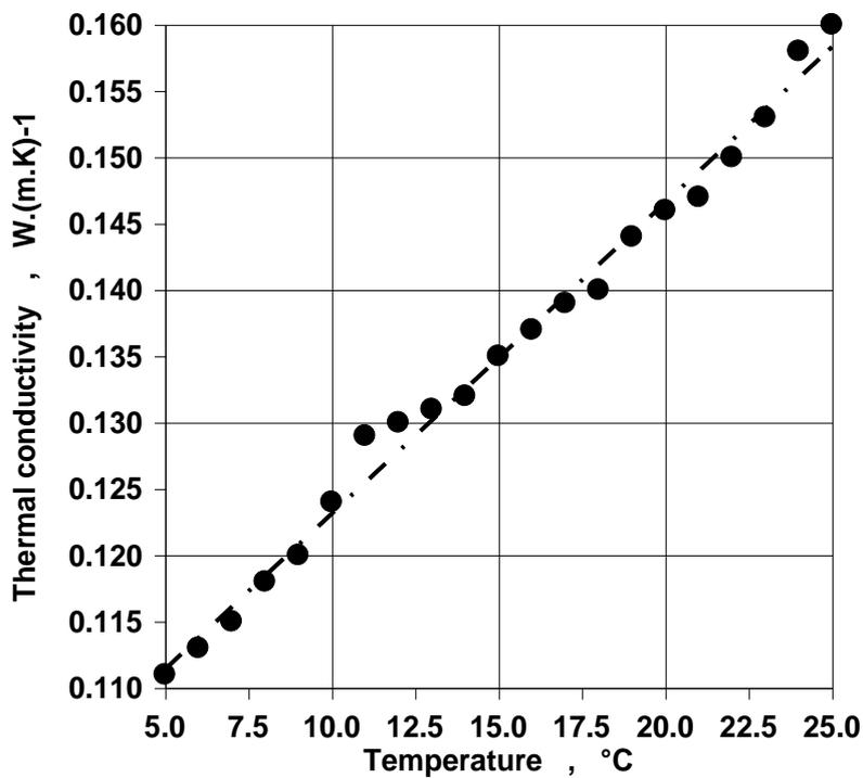
**Figure 5** Relation of perga thermal conductivity to temperature during the temperature stabilisation in temperature range (5 – 25) °C
