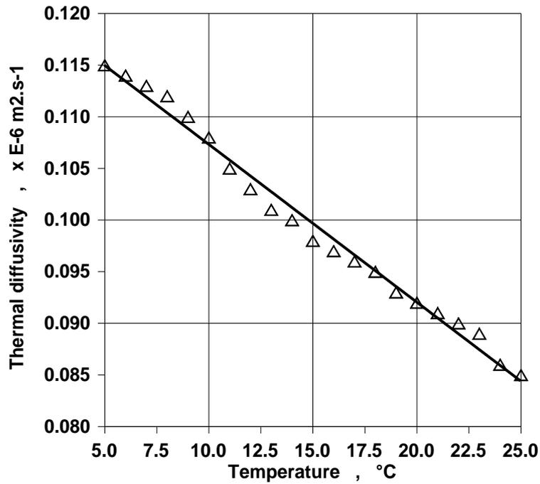
**Figure 2 Relation of honey thermal diffusivity to temperature during the temperature stabilisation in temperature range (5 – 25) °C**
