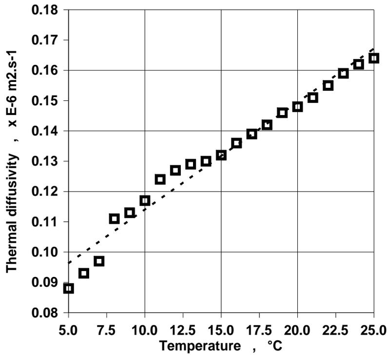
**Figure 4** Relation of granular bee pollen thermal diffusivity to temperature during the temperature stabilisation in temperature range (5 – 25) °C
