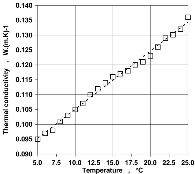
**Figure 3 Relation of granular bee pollen thermal conductivity to temperature during the temperature stabilisation in temperature range (5 – 25) °C**
