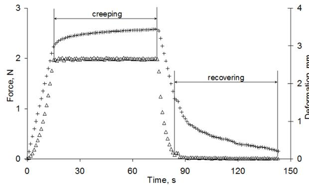
Fig. 1. Typical CRT curve measured on gum candy
