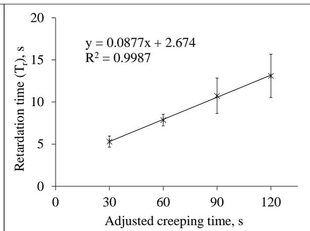
Fig. 4. Change of retardation time (average  $T_r$  with standard deviation) of four elements Burgers-model with stretched exponent as the function of creeping time
