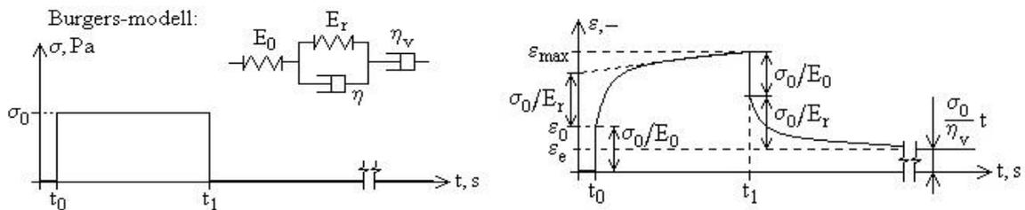
Fig. 2. The four elements Burgers-model and the meaning of model parameters in CRT curve (based on SITKEI (1981))
