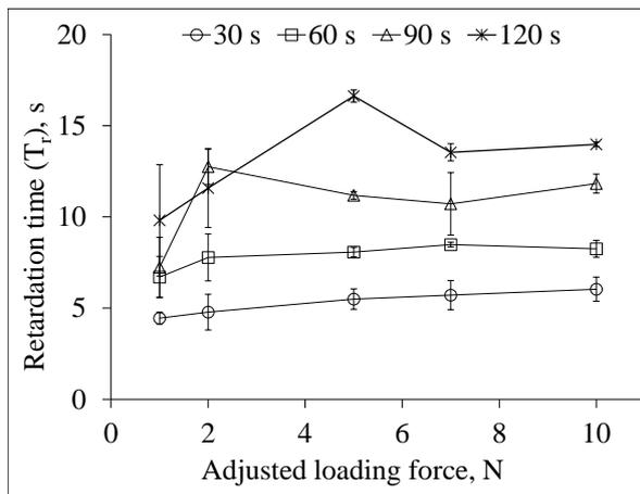
Fig. 3. Change of retardation time ( average  $T_r$  with standard deviation) of four elements Burgers model with stretched exponent as the function of loading force
