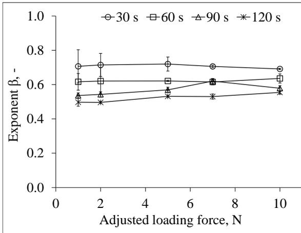
Fig. 5. Change of stretch exponent (average  $\beta$  with standard deviation) of four elements Burgers-model as the function of loading force
