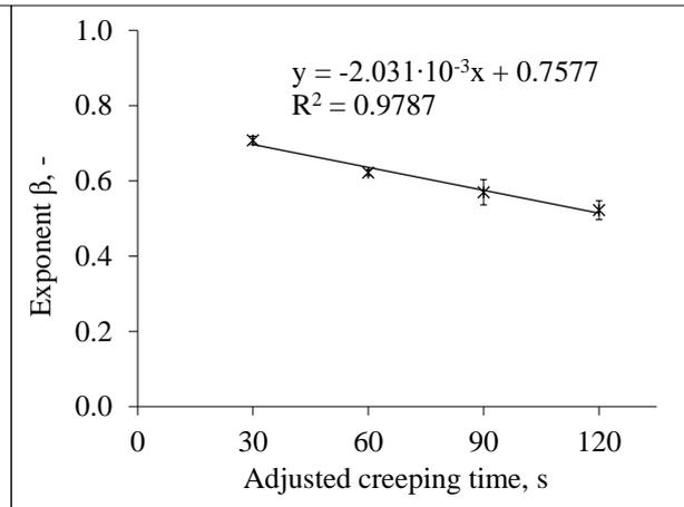
Fig. 6. Change of stretch exponent (average  $\beta$  with standard deviation) of four elements-Burgers model as the function of creeping time
