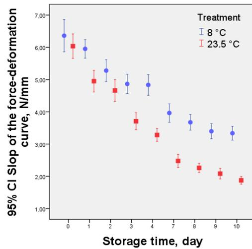
Fig. 2: The changes of the slope of the force-deformation curve during the storage period
