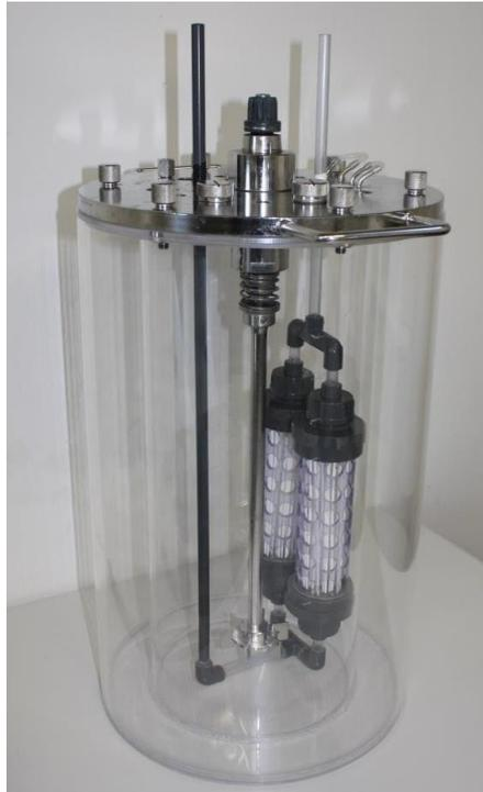
Figure 1: STR equipped with membrane modules
