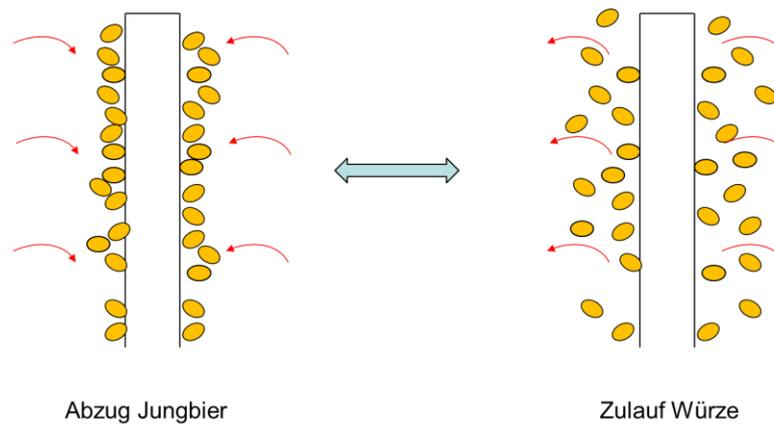
Figure 2: Alternating operation of the membranes
